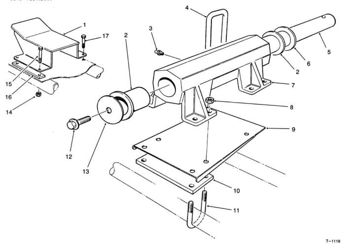
FIXED HEAD INSTALLATION FOR CUTTING UNIT NO. 2 (L. H.) & NO. 3 (R. H.)
